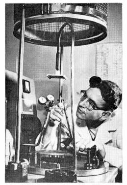
A PATENT has been issued for this apparatus, invented by D. M. Mattox (1123), which makes possible ion plating of numerous metals which could not be coated by conventioinal techniques.
